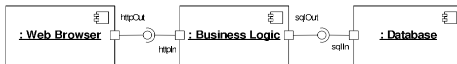
Figure 10. A UML 2.0 component diagram depicting the structure of a simple Web application
