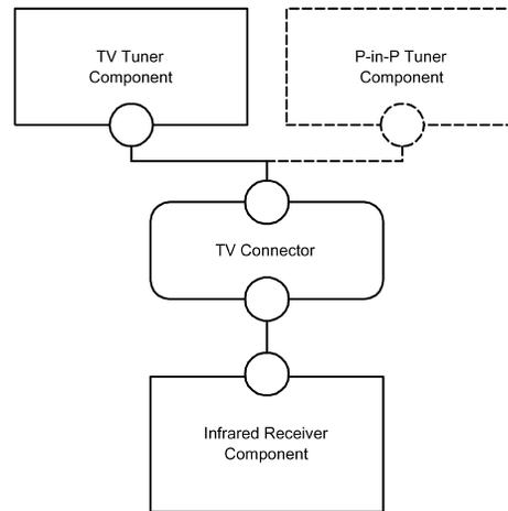
Fig. 8. Diagram for a television product-line where the picture-in-picture elements are optional, accompanied by xADL 2.0 description.
